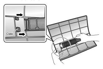
2. Clean or replace the titanium apatite photocatalytic airpurifying filter.
